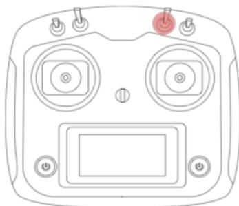
The flight speed can be adjusted using the toggle key [CH7(SwC)] of the controller.
