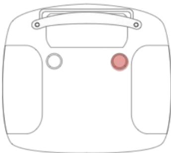
After starting in altitude hold mode, release throttle and short press toggle key1 (CH9) on the back to take off. Short press toggle key1 (CH9) again to landing. After landing, the motor can be stopped using toggle key [CH8 (SwD)].
