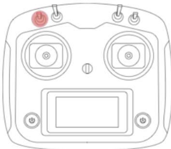
The mode can be set using toggle key [CH5(SwA)].
