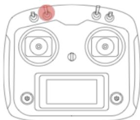
\*The headless mode can be turned on and off using the toggle key [CH6(SwB)].
