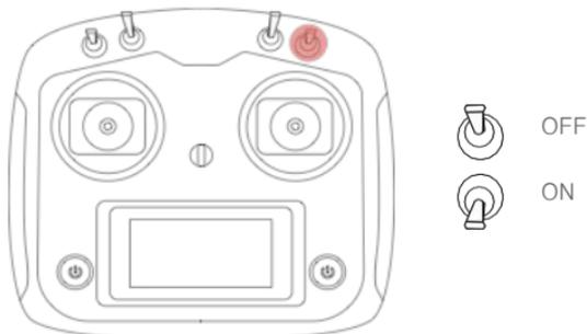
The motor can be stopped using toggle key [CH8(SwD)] as indicated. Stop the motor in the event of a dangerous situation as it can be stopped under any circumstances.
