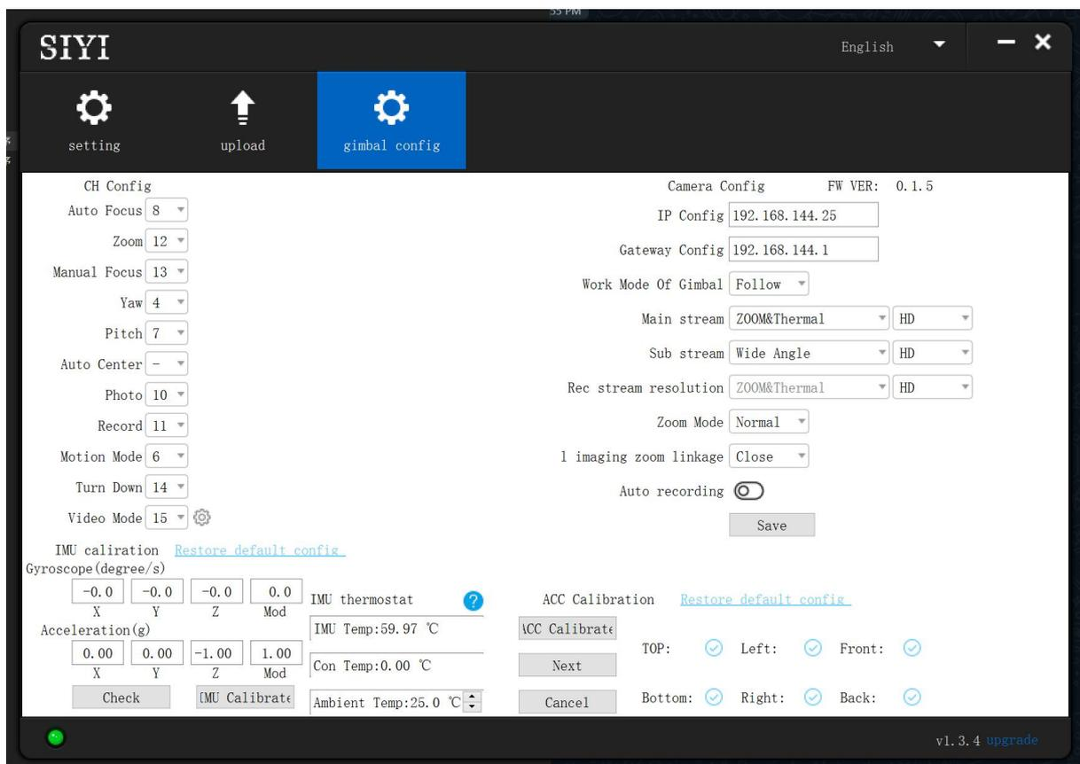
7. Under "Channel Config" page, assign the communication channel 1 to 16 to target gimbal and camera functions according to your requirement.
