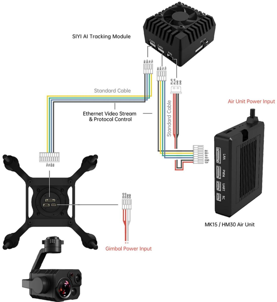
4. Please refer to the picture below to connect SIYI gimbal camera with flight controller and integrate attitude data.
